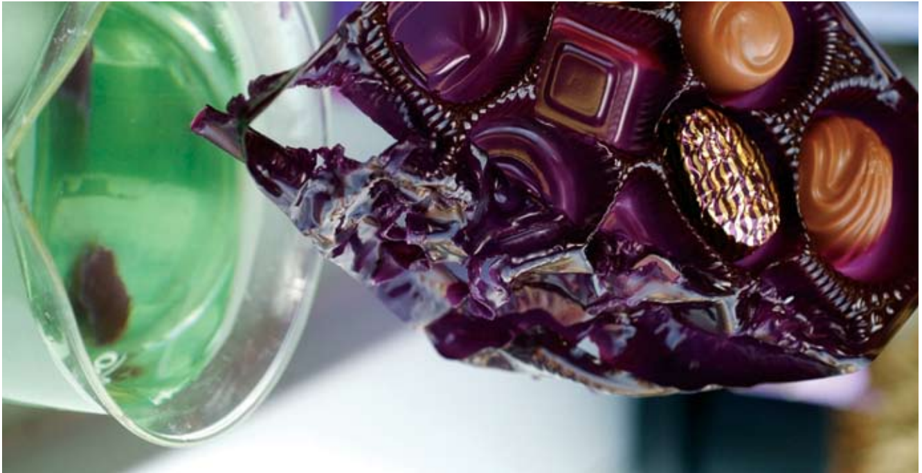
A water-soluble, biodegradable plastic for food packaging has been developed and produced in Australia by the CRC for International Food Manufacture & Packaging Science and Melbourne-based start-up company Plantic Technologies. Cadbury is using the product for its Milk Tray range of boxed chocolates, and Swinburne's Professor Greg Lonergan and Dr Ranjith Jayasekara are testing its biodegradability.
