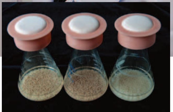
Pictured above: Samples of POP-inhibiting fungus immobilised in hydrogel-beads, grown in the Swinburne Sarawak lab.
